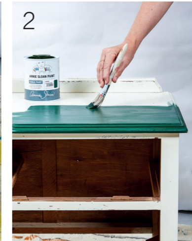
2 Paint the unit with two coats of Amsterdam Green, letting the paint dry between coats.
