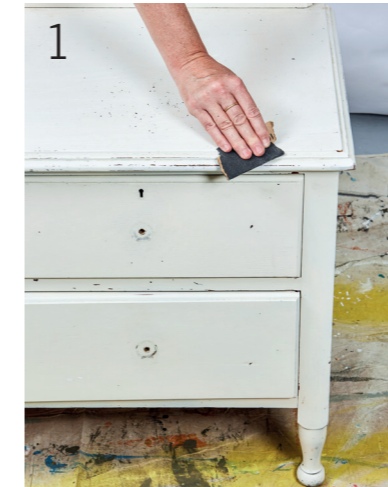
1 Remove the handles from the drawers and then lightly sand all the surfaces.
